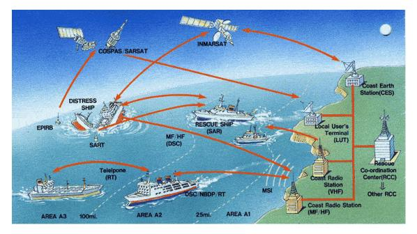
**PRESCOM** especially offers GMDSS Digital selective calling (DSC) solutions to Coast Authorities and commercial radio communication Operators in the A1, A2, A3 & A4 areas. The solution may be offered both for the GMDSS and the commercial services either in manual and or in automatic for the VHF, MF and HF frequency bands.
